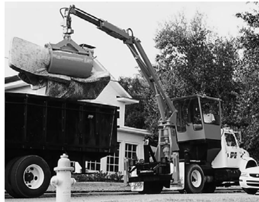
A brush truck lifts bulky items into a dump bed for disposal at a landfill.
