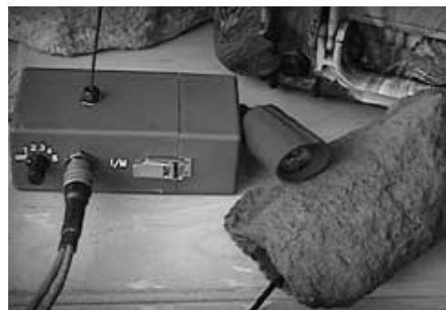
Sensors placed near the dumpsite trigger a device to begin recording.
