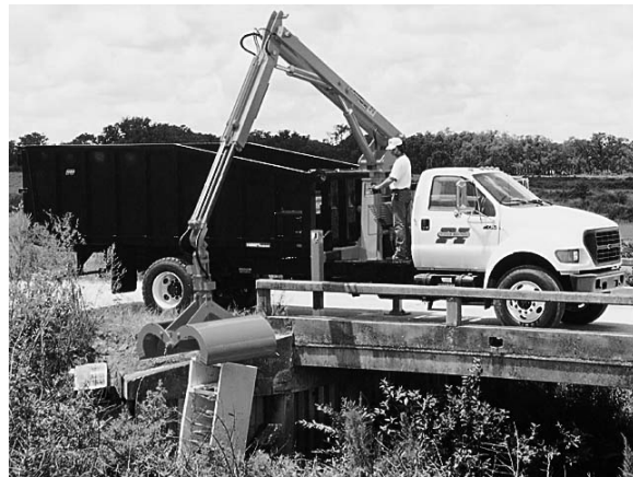
A brush collection vehicle is used here to lift illegally dumped materials out of a ravine.
